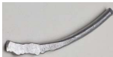
Solder sample prepared for testing.
