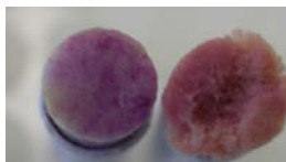
Blank swab on left; test swab on right immediately after test.
